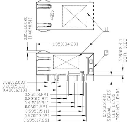
7. THE PART IS COMPLIANT WITH WAVE SOLDERING, THE SUGGESTED PEAK WAVE SOLDERING CONDITION IS 260°C MAX. AND 10 SECONDS MAX..
