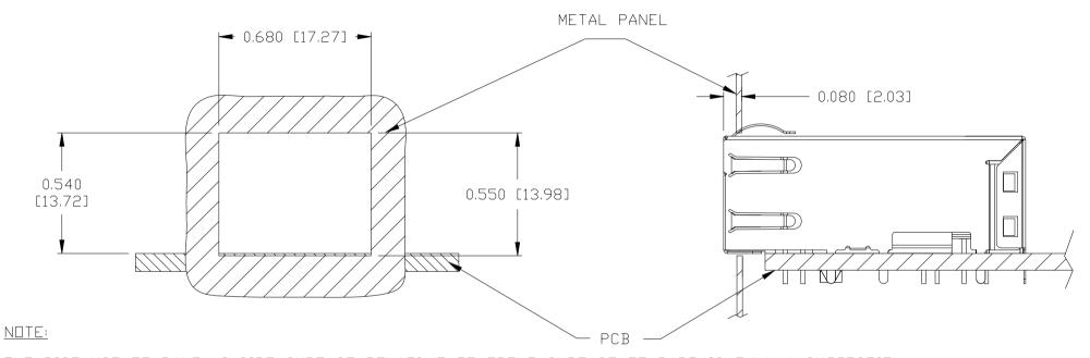
THE DISTANCE OF PANEL INSIDE SURFACE RELATIVE TO FRONT SURFACE OF PART IS ONLY A SUGGESTION. IN CASE THIS DISTANCE IS DIFFERENT, THE REQUIRED PANEL OPENING DIMENSIONS CHANGE ACCORDINGLY.
